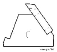
The knives can be sharpened only as much as is shown in the adjacent figure. After that, they are worn out and should be replaced by new ones in order for the granulation to be effective.
